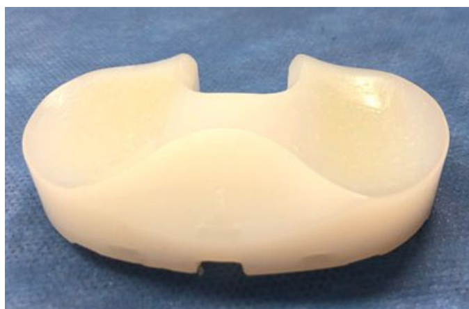
Figure 2: Left polyethylene component shows mild wear.
